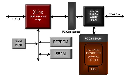
Figure 4: Block Diagram of UART to PC Card (PCMCIA) Bridge
