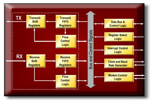
Figure 2: Standard UART Functional Blocks
