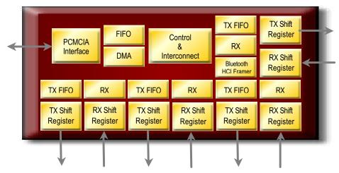
Figure 7: Functional Blocks of PC Card (PCMCIA) to Multiple UARTs Bridge
