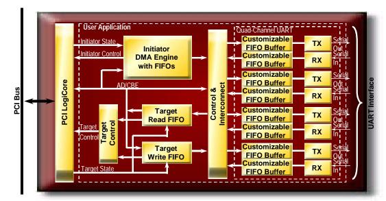
a 16 byte FIFO, which could easily support FOUR simultaneous 721 Kbps maximum data rate Bluetooth connections.
