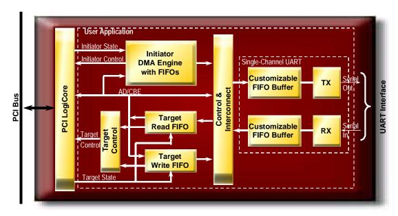
Figure 5: Single-Channel UART to PCI Bridge
