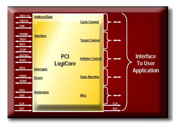
Figure 3: The PCI LogiCore Block
