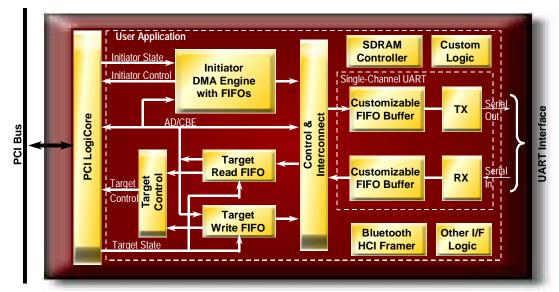
Figure 7: Single-Channel UART to PCI Bridge with Added Functionality
