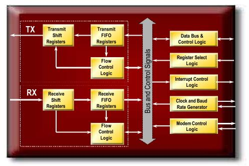
Figure 2: Standard UART Functional Blocks
