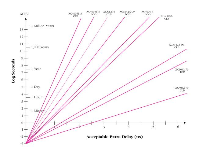
**Figure:** Mean Time Between Failure for various IOB and CLB flip-flop outputs when synchronizing a 1 MHz asynchronous input with a 10 MHz clock. XC4005E-3 and the XC3142A-09; and, for comparison purposes, two older-technology devices, the XC4005-6 and the XC3042-70. In each device, two different implementations test the IOB and CLB flip-flops. The XC5200-5 CLB flip-flop was also tested. (There is no IOB flip-flop in XC5200 architecture.)
