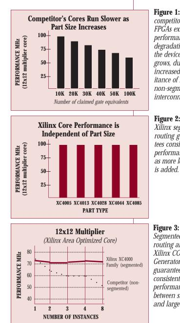
Figure 1: Our competitor's FPGAs exhibit performance degradation as the device size grows, due to the increased capacitance of long non-segmented interconnections.
