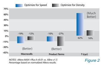
**Results** - As shown in **Figure 1**, XC9500 CPLDs use 18% fewer macrocells, 9% fewer product terms, and achieve an 8% faster clock frequency than Altera MAX7000S devices. As shown in **Figure 2**, XC9500XL CPLDs use 19% fewer macrocells and 10% fewer product terms, and achieve an impressive 62% faster system performance than Altera's MAX7000A/AE products.
