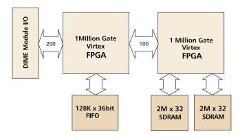
Nallatech's range of DIME motherboards and modules enable you to rapidly develop custom applications without the need to design and manufacture custom PCB's. at the turn of the century we could squeeze over 2.2 Million programmable logic gates, 16-Mbytes of memory, and a 4-Mbit FIFO into a few square inches?
