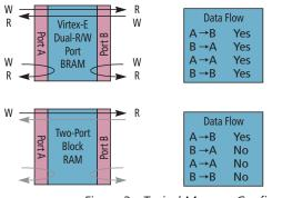
Figure 3 - Typical Memory Configurations
