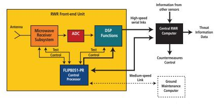
Figure 1 - Radar Warning Receiver (RWR) system.
