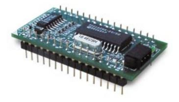
Figure 1 - Configurator 32-pin DIP module.
