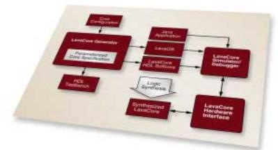
Figure 3 - LavaCORE design environment.
