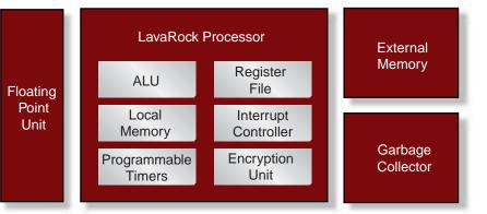
Figure 2 - LavaCORE system architecture.
