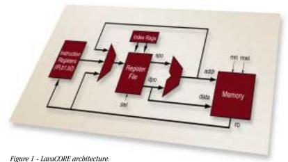
A 16x32-bit dual-ported RAM implements the register-file. The instruction register is composed of three 8-bit registers denoting the instruction, byte one, and byte two of the instruction stream. A 32-bit ALU computes arithmetic and logical operations. Additional signals include clock, reset, signal interrupt, memory interface, and a set of observability pins for the state and flags.
