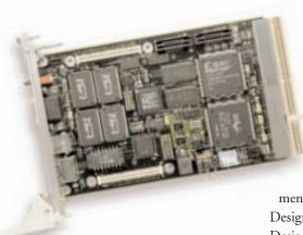
A StrongArm SA1110 Processor provides the processing power and a Xilinx Spartan-II XC2S100 implements a glueless interface between the SA1110 processor bus and the industry standard PCI bus. Along with these hardware resources, Avnet Design Services provides IP cores for PCI,
