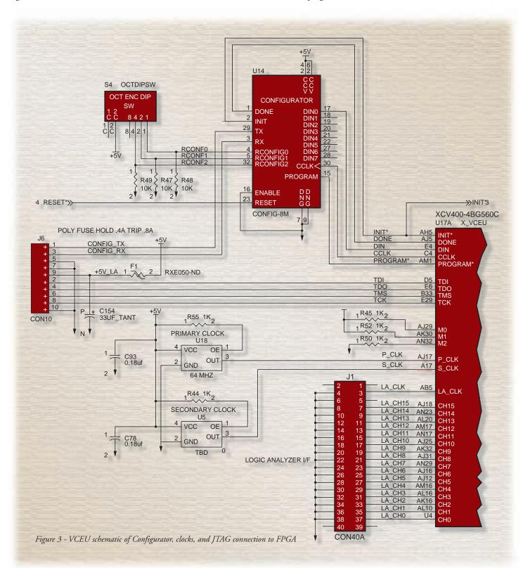
The front panel of the VCEU card has an octal encoded rotary switch that connects to the Configurator and selects one of eight possible bitstreams to be loaded into the XCV400. In addition, the Configurator module's RS232 signals are connected to the VME front panel for easy downloading of new bitstreams from a field service laptop or any other device with a serial port. The VCEU card schematic of the Configurator interface is shown in Figure 3.
