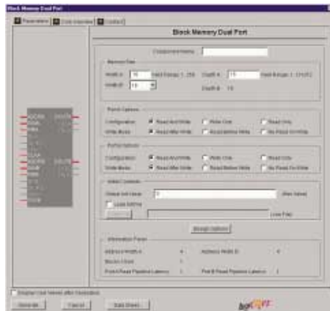
Figure 1: Parameterization window for the Dual Port Block Memory LogiCORE
