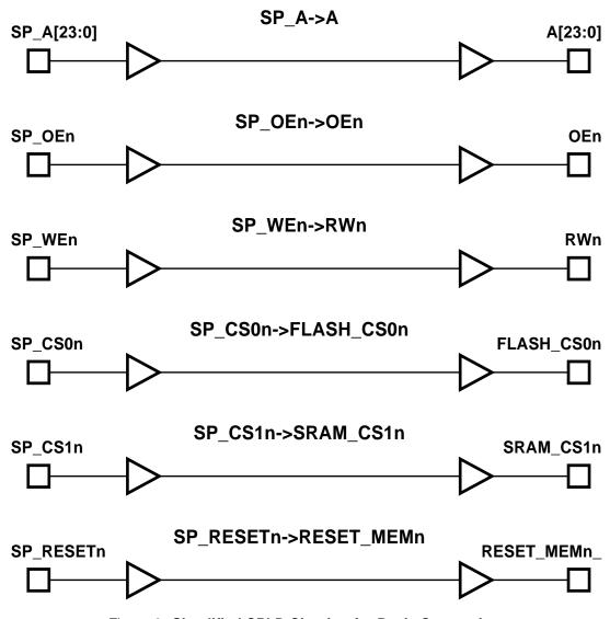
Figure 6: Simplified CPLD Circuitry for Basic Connections
