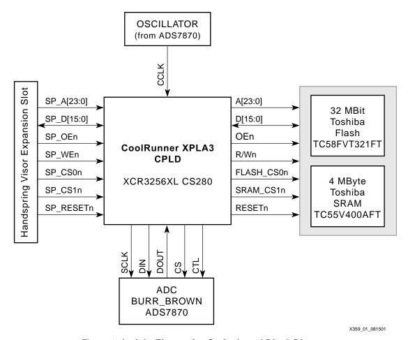
Figure 1: Insight Electronics Springboard Block Diagram
