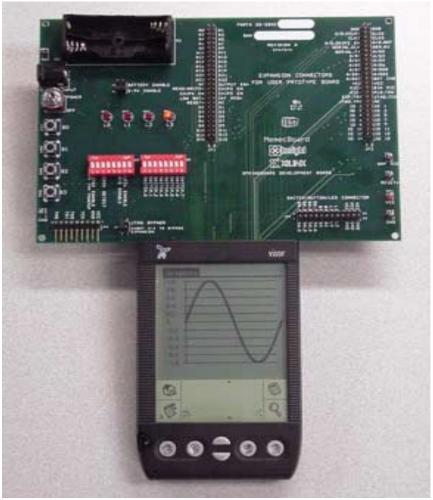
Figure 3: Insight Circuit Card Inserted into Visor
