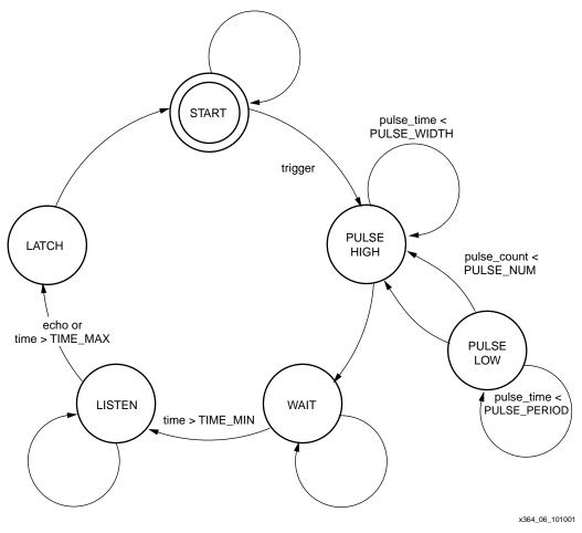
Figure 6: Measurement State Machine
