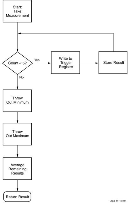
Figure 8: SB\_TakeMeasurement Flow Chart
