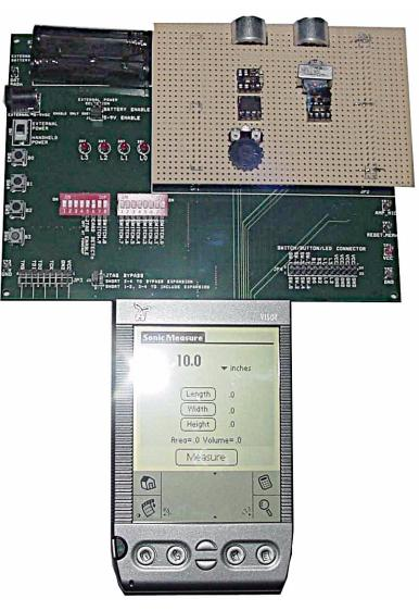
display the measured distance in the desired measurement unit. Figure 1 shows the Sound Bouncer module operating together with the Handspring Visor.
