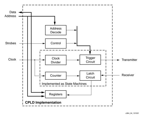
connector to the flash memory. Figure 4 shows the CPLD functional block diagram for the Sound Bouncer design.
