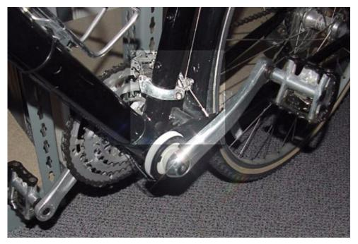
the periodic output of the sensor. Figure 7 below shows the cadence sensor mounted on the bicycle's crank.
