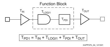
Figure 4: T<sub>PD1</sub> with a Single Product Term
