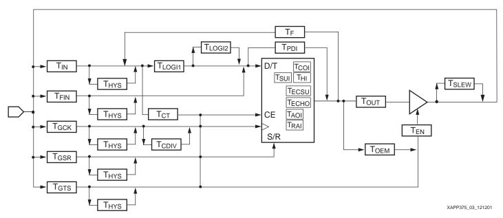
Figure 3: CoolRunner-II Timing Model
