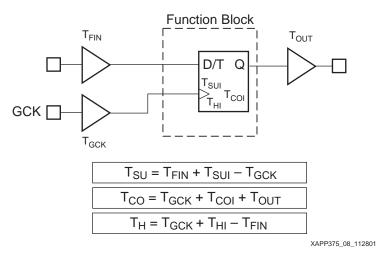
Figure 8: Fast Input Register Path
