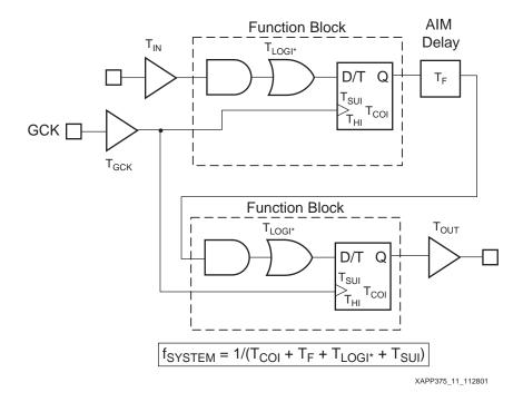
Figure 11: Multiple Logic Levels
