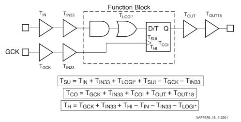
Figure 15: I/O Standard Timing Example
