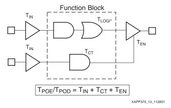
Figure 13: Product Term Output Enable Timing
