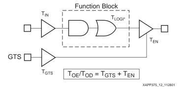
Figure 12: Global Output Enable Timing
