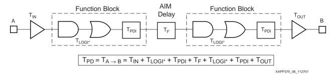
Figure 6: T<sub>PD</sub> with Two Levels of Logic
