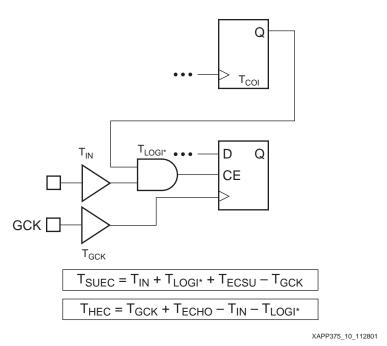
Figure 10: Clock Enable Timing Parameters
