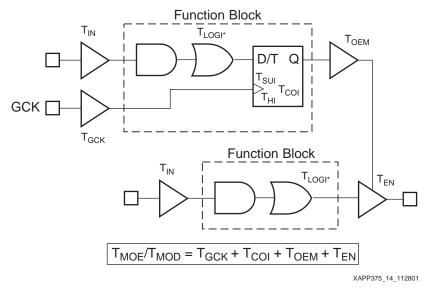
Figure 14: Macrocell Driven Ouput Enable Timing
