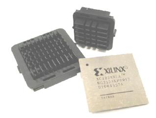
Figure 7: Enhanced BGA with Low Profile Retainer Type Passive Heatsinks
