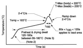
Figure 3: Typical Conditions for IR Reflow Soldering
