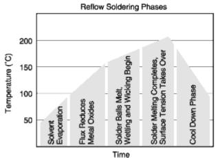
Figure 1: Soldering Sequence
