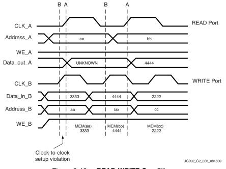
Figure 2-46: **READ-WRITE Conditions**
