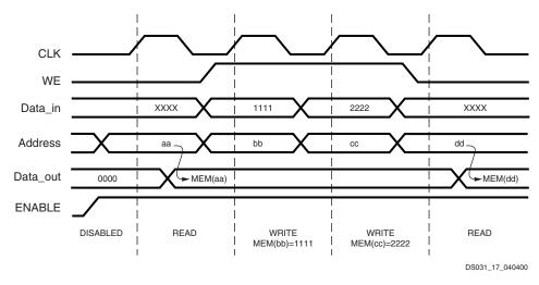
Figure 2-45: NO\_CHANGE Mode Waveforms
