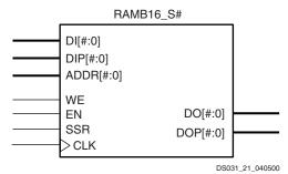
Figure 2-48: Single-Port Block RAM Primitive
