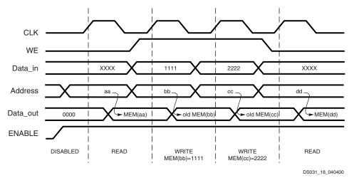
Figure 2-44: **READ\_FIRST Mode Waveforms**
