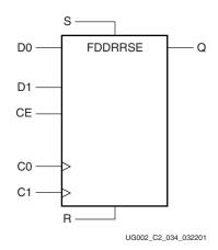
Figure 2-114: FDDRRSE Symbol: DDR Flip-Flop With Clock Enable and Synchronous Reset and Set
