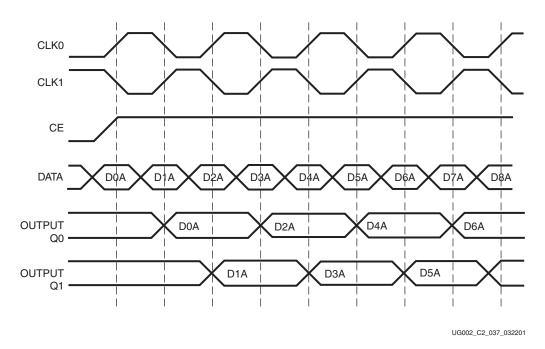
Figure 2-109: Input DDR Timing Diagram
