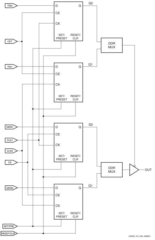
Figure 2-112: Output DDR With 3-State Control
