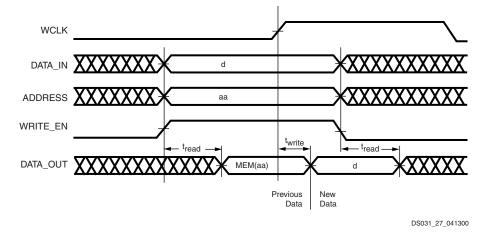
Figure 2-50: Write Timing Diagram
