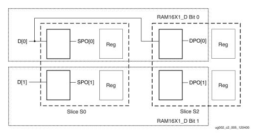
Figure 2-53: Two RAM16X1\_D Placement
