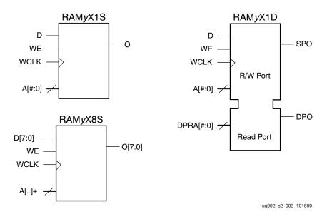
Figure 2-51: Single-Port and Dual-Port Distributed SelectRAM Primitive
