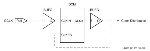
Figure 2-4: Clock Distribution with DCM
