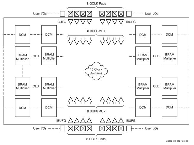
Figure 2-1: Clock Resources in Virtex-II Devices
