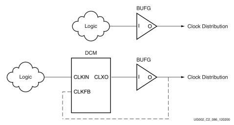
Figure 2-5: Internal Logic Driving Clock Distribution
