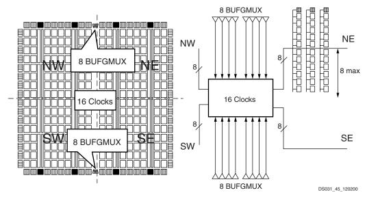
Figure 2-11: Clock Buffer Outputs per Quadrant
