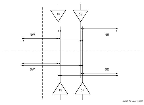
Figure 2-7: Facing BUFG#P and BUFG#S Connections
