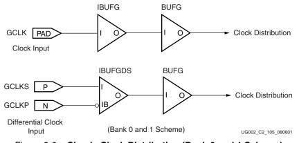
Figure 2-2: Simple Clock Distribution (Bank 0 and 1 Scheme)
