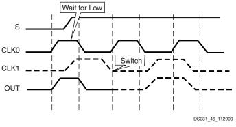
Figure 2-17: BUFGMUX Waveform Diagram
