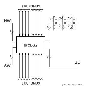
Figure 2-13: Low-Power Clock Network
