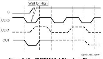
Figure 2-18: BUFGMUX\_1 Waveform Diagram
