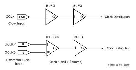
Figure 2-3: Simple Clock Distribution (Bank 4 and 5 Scheme)
