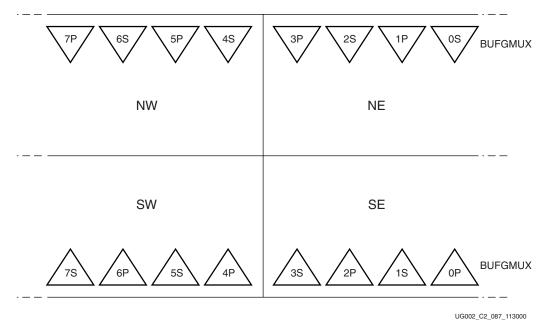
Figure 2-6: Primary and Secondary Clock Multiplexer Locations
