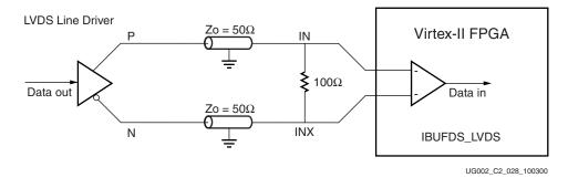
Figure 2-117: LVDS Receiver Termination
