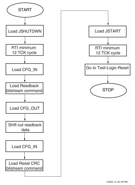
Figure 3-36: Regular Readback Flow
