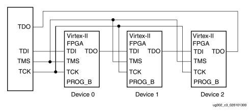
Figure 3-25: Boundary Scan Chain of Devices
