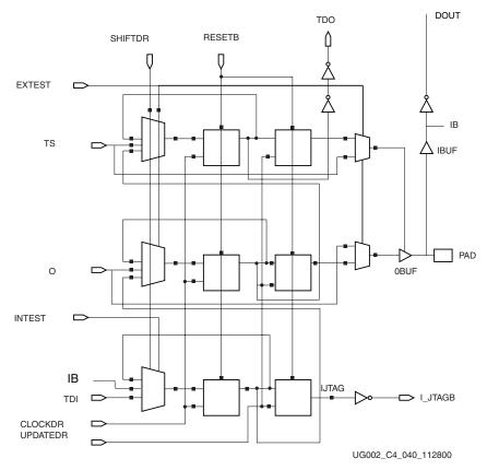
Figure 3-21: Virtex Series Boundary Scan Logic
