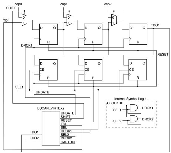
Figure 3-22: BSCAN\_VIRTEX2 (Example Usage)
