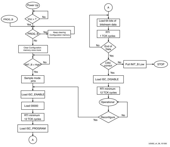
Figure 3-27: IEEE 1532 Configuration Flow
