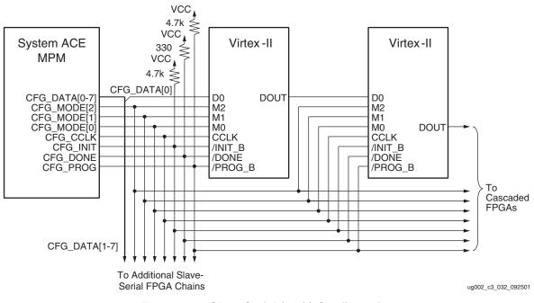
Figure 3-7: Slave Serial (1-bit) Configuration
