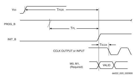
Figure 3-2: Power-Up Timing Configuration Signals
