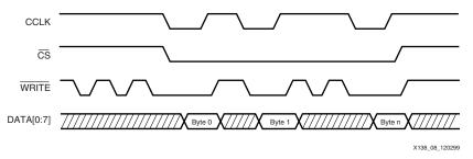
Figure 3-19: Controlling CCLK for RDWR\_B De-Assertion
