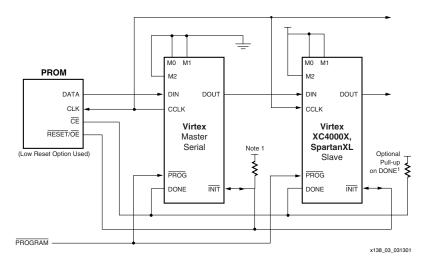
Figure 3-12: Master/Slave Serial Mode Circuit Diagram
