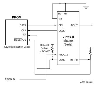
Figure 3-10: Master Serial Mode Circuit Diagram
