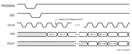
Figure 3-11: Master Serial Configuration Cloaking Sequence
