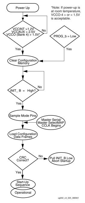
Figure 3-1: Configuration Process
