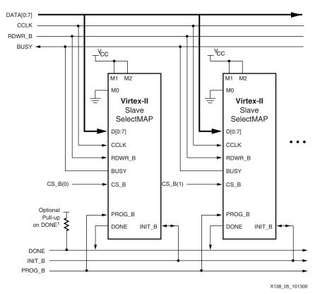
Figure 3-16: Slave SelectMAP Mode Circuit Diagram
