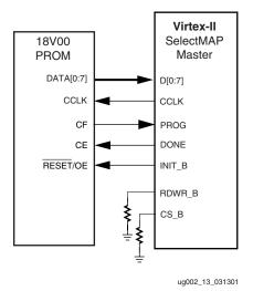
Figure 3-14: Virtex-II Interfaced With an 18V00 PROM
