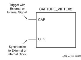
Figure 3-35: Readback CAPTURE\_VIRTEX2 Library Primitive
