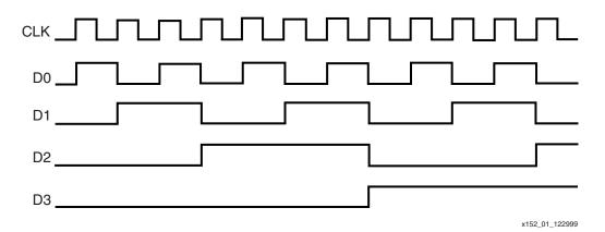
Figure 4-68: Output Waveform of a 4-bit Counter
