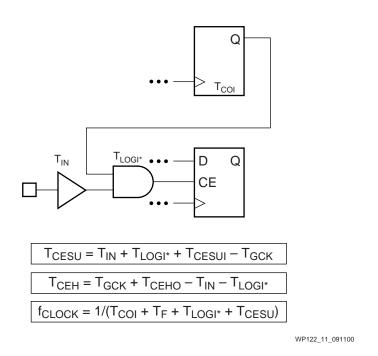
Figure 11: Flip-Flop with Clock Enable
