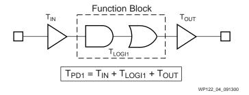
Figure 4: T<sub>PD1</sub> with a Single Product Term
