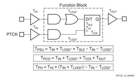
Figure 10: Single Flip-Flop with Product Term Clock
