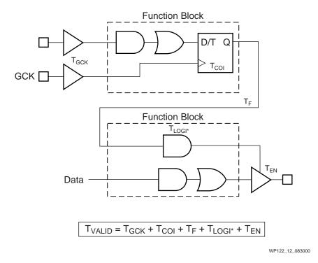
Figure 12: Flip-Flop-Controlled Output Enable
