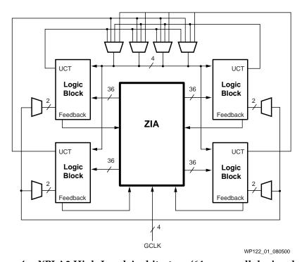
Figure 1: XPLA3 High-Level Architecture (64 macrocell device shown)
