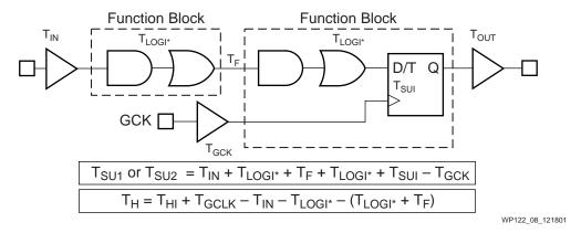
Figure 8: Flip-Flop with Two-Pass Logic
