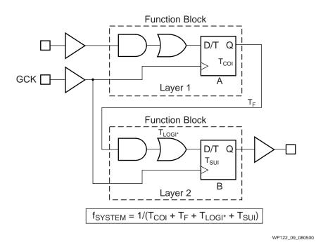
Figure 9: Multiple Flip-Flops with Single Level Logic
