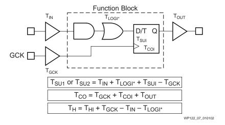
Figure 7: Simple Flip-Flop Path
