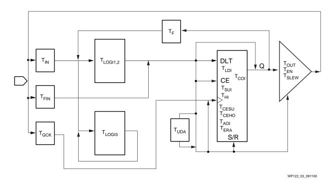
Figure 3: XPLA3 Detailed Timing Model
