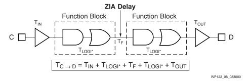
Figure 6: T<sub>PD</sub> with Two-Pass Logic
