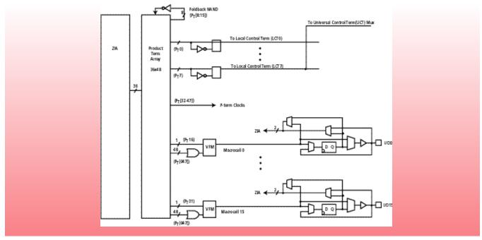
Figure 2 - XPLA3 Logic Block architecture.
