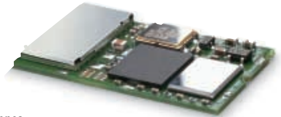
Figure 1 - Ericsson Bluetooth transceiver module
