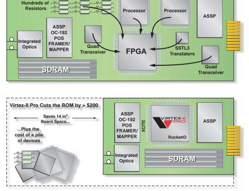
Figure 1 - Leading edge price/performance through integration and reduction of board size
