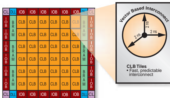
Figure 8 - FPGA CLBs and interconnect resources
