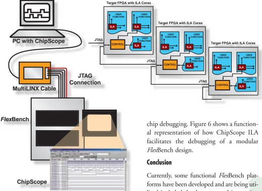
Figure 6 - ChipScope and FlexBench solution
