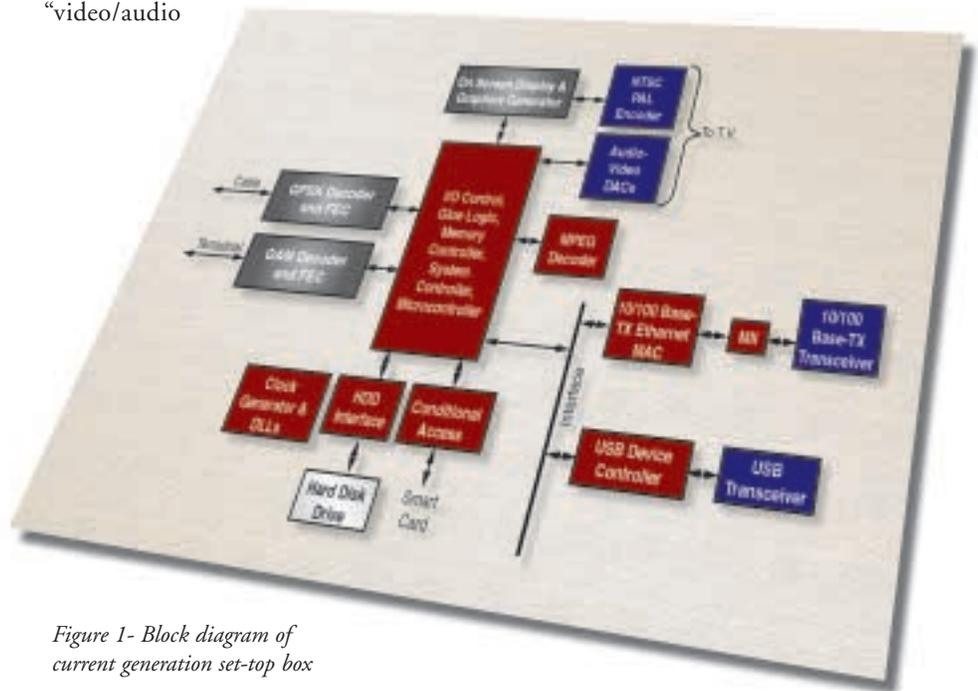
Figure 1- Block diagram of current generation set-top box
