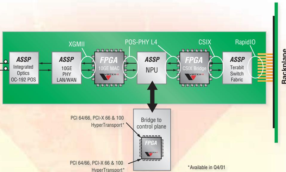
Figure 3 - 10-Gigabit Ethernet LAN/WAN card application example
