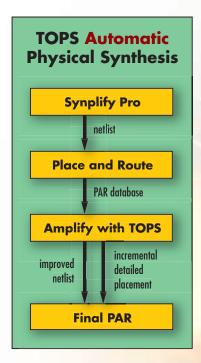
Figure 1 - Automatic physical synthesis using TOPS
