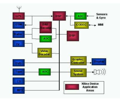
Figure 3 – Typical Elements of an Infotainment System
