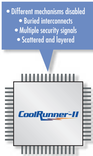
Figure 2 - Multiple security functions embedded in CoolRunner-II CPLD
