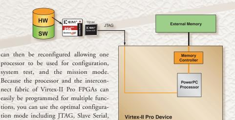
Figure 2 - Configuration via JTAG port
