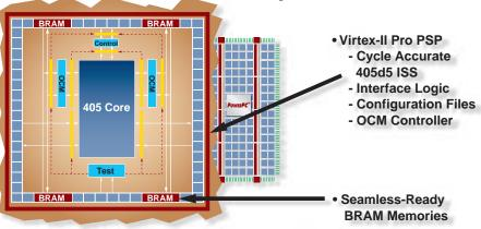
Processor Block = CPU Core + Interface Logic + Immersion Tiles
