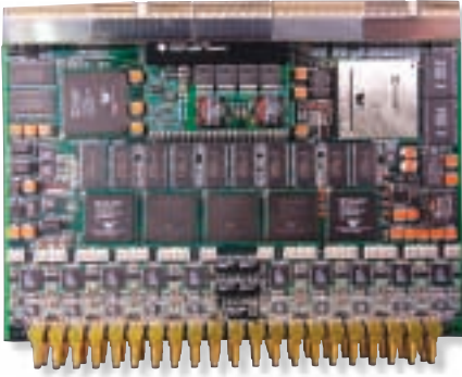
Figure 7 - Xilinx Virtex-E FPGAs on a BenADIC 20-channel, 14-bit data acquisition card
