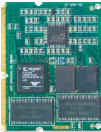
Figure 4 - Virtex XC2V1000 implemented on Hitachi SH4 \mu Engine
