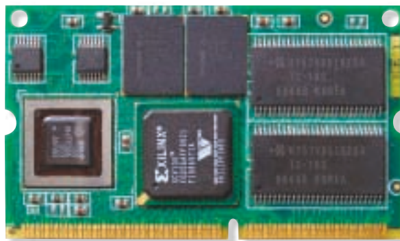
Figure 3 - Hitachi SH3 \mu Engine with Virtex XCV100
