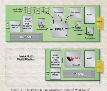
Figure 3 - The Virtex-II Pro advantage: reduced PCB board space with less complexity and fewer components
