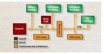
Figure 5 - Hard and soft IP cores
