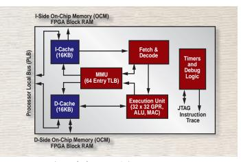
Figure 4 - Inside the PowerPC 405 processor
