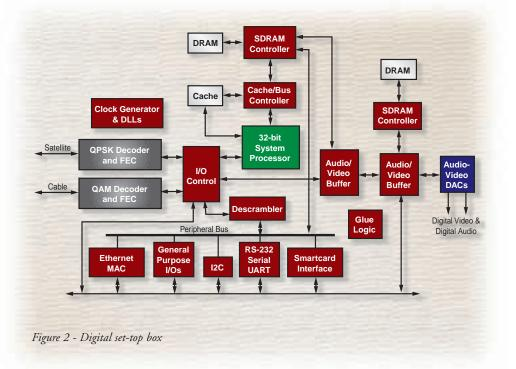
that is, it contains a Web browser (which is really a Hypertext Transfer Protocol (HTTP) client) and the Internet's main program, TCP/IP. The service to which the set-top box is attached may be through a telephone line or through a cable TV company.
