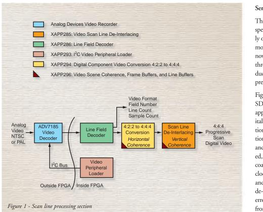
it to progressive-scan, 4:4:4 component digital video in a series of steps. An Analog Devices ADV7185 video decoder converts the analog video to digital video. The other conversion steps are implemented in the Virtex-II FPGA.
