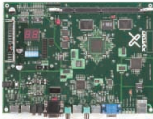
Figure 2 - Xyron Semiconductor Edison development board incorporates a Xilinx Virtex-II XC2V1000 FPGA.
