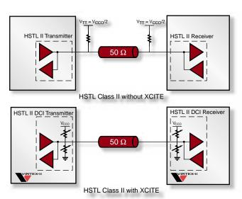
Figure 1 - Termination resistors on-chip
