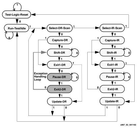
Figure 3: Test Access Port State Diagram
