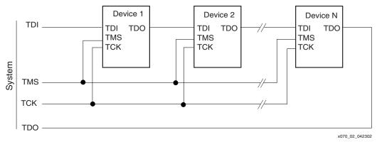
Figure 2: Single-Port Serial Boundary Scan Chain
