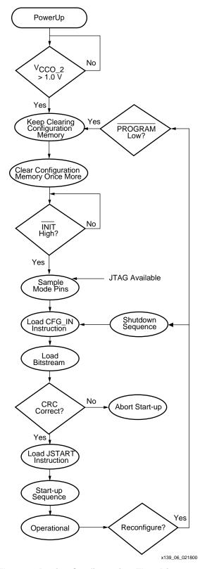
Figure 6: Device Configuration Flow Diagram
