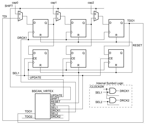
Figure 4: BSCAN\_VIRTEX (Example Usage)
