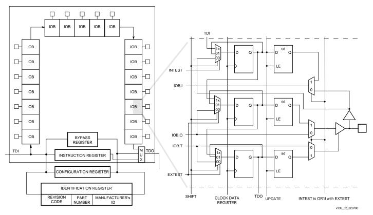
Figure 2: Virtex Series Boundary Scan Logic
