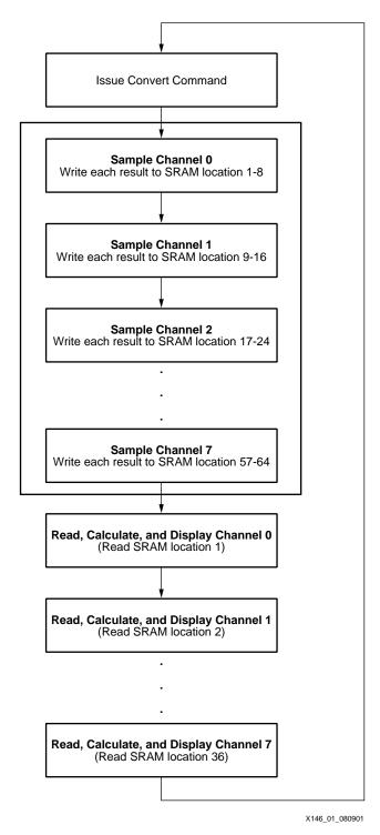
Figure 1: Operational Flow of Digital Volt Meter Design
